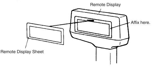
Affix the remote display sheets to the depressed area of the remote display on both sides. (Operator side and customer side)
